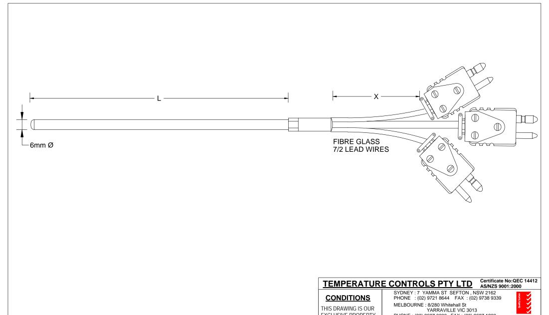
TYPE K THERMOCOUPLE TRIPLEX ASSEMBLY **COMPLETE WITH LARGE PLUGS**  **EXCLUSIVE PROPERTY** AND MUST NOT BE COPIED OR HANDED TO ANY OTHER PARTIES WITH OUT WRITTEN PERMISSION. IT SHALL BE RETURNED UPON **REQUEST**
